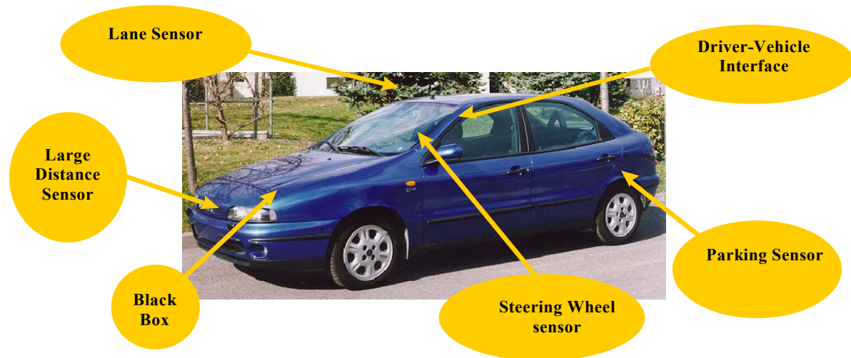
Picture 9: Natural architecture of the sensors in an equipped research vehicle
